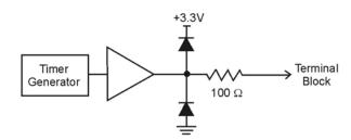
Figure 23. Typical USB-1616HS-2 timer channel
